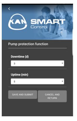
**Pump protection feature** – allows to set the time the pump deactivation in days or the working time in minutes.
