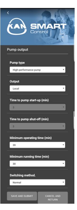
**Pump type** – the choice of the system pump: Conventional pump or high performance pump (energy-saving).
