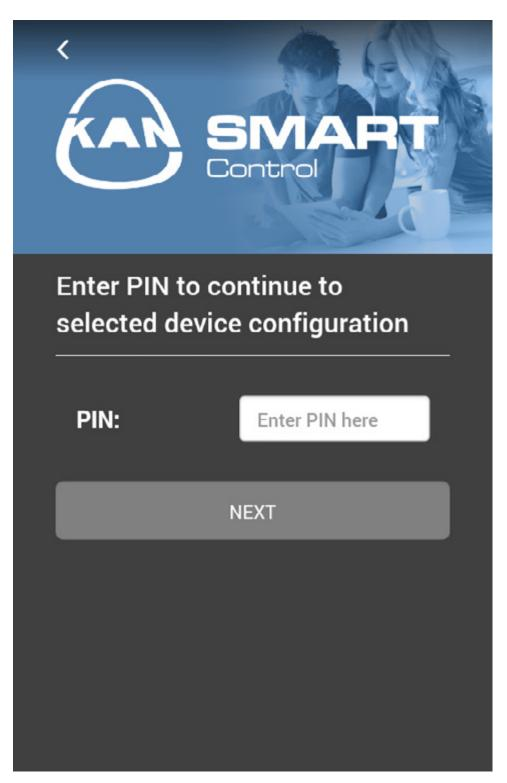
The administrator's panel is protected by a PIN code. The default PIN code is 1234. Be aware that the changes made in the administrator panel may have an impact on the correct operation of the heating and cooling installation. The changes should be made after reading the electric terminal block Manual and EZR-manager program.
