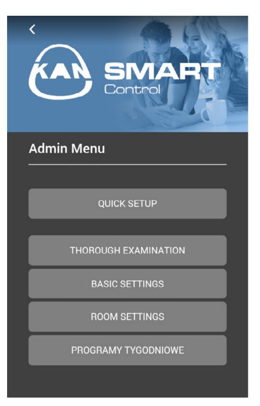
Quick setup – allows to configure the terminal blocks quickly and set the basic functions.
