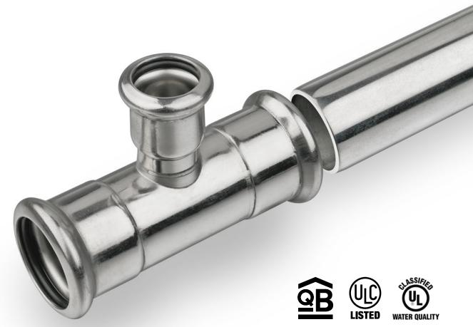
SYSTEM KAN-therm Steel is an installation system consisting of pipes and fittings made of zinc-plated carbon steel with diameters range 12 up to 108 mm, which are connected by means of radial press technique.
